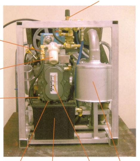
BLOWER OIL DRAIN WATER HOLDING TANK 2909886
